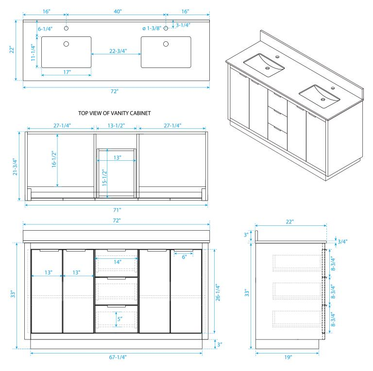
\*Note: Due to high probability of breakage, the backsplash comes in two pieces, cut from the same piece. All measurements are ±1/4".
